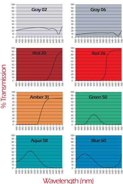
TSP color filters are available in a wide range of standard colors in both acrylic and polycarbonate. These filters are designed for use with the most commonly used displays (LCD, LED, EL, VF, etc.). TSP can also prepare filters colormatched to specific application requirements or to duplicate the color of existing filters. Choosing the proper color will provide sharp, high resolution characters with enhanced contrast between the displayed information and the background.
